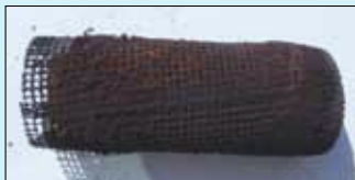
Used strainer with clogged mesh, needs to be replaced.
